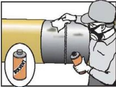
3. Insure that surfaces are clean of grease, oil, salts and other contaminants. If necessary, use Acetone, MEK or other suitable solvent. Perform cleaning when pipe is 3°C (5°F) above dew point.
