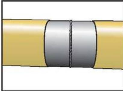
5. A 2.5-4 mil (63.5-101.6 micron) surface profile with sharp angularity. Burnishing or polishing must be avoided. Surface preparation can be controlled using surface profile tape. Dry surface and insure ideal surface preparation.
