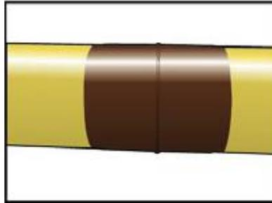
12. The curing rate\* will vary according to pipe and ambient application temperature. Refer to curing rate chart to determine when to perform a Shore D check.
