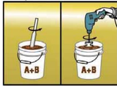
8. Use a mixing speed that uniformly blends the 2 parts, but does not create a vortex in the mixture or spillage.
