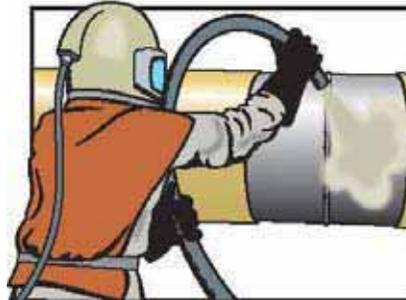
4. Blast clean surface to a near white ISO-8501, NACE No. 2, SA-2 1/2 (SSPC-SP 10) or better using particle blasting (sand or other). Sweep blast adjacent FBE coating 50 mm (2") to either side of bare steel area (cutback).
