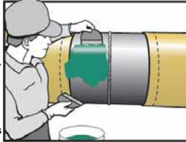
10. Use trowel, brush or roller to apply required minimum thickness of coating. Cover at least 50 mm (2") of the adjacent mainline coating.
