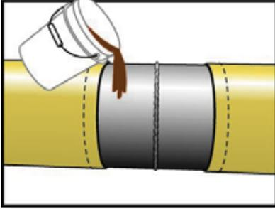
9. Reconfirm that the application temperature is above 10°C (50°F)\* & 3°C (5°F)\* above the dew point. Then slowly pour mixed epoxy onto pipe. See "Tips" below for additional suggestions.
